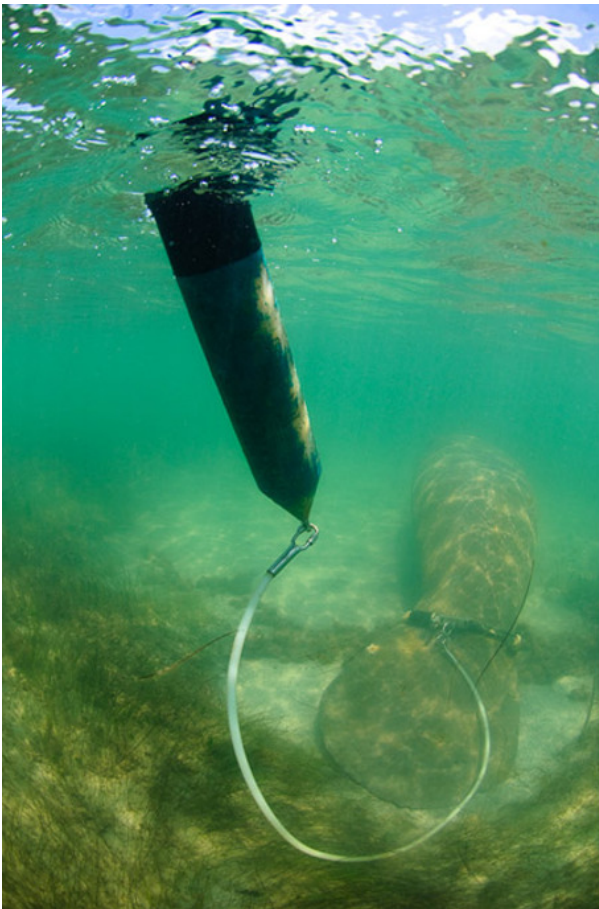
Left: Manatee with tagging equipment (peduncle belt, a flexible tether and a floating transmitter. Photo: Luciano Candisani/Aquatic Mammals Foundation Collection. Right: VHF telemetry receivers used in manatee tracking. Photo: Aquatic Mammals Foundation
